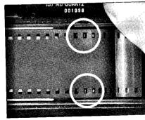
[6] Take additional dummy exposures until "1" appears in the exposure counter (this can also be verified using the counter visible on the left inside the viewfinder). Now you can start taking pictures. When taking the dummy exposures, make sure that the film feed indicator on the camera back is turning. This indicates that the film is feeding properly. The rewind knob will turn at the same time.
