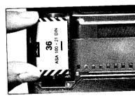
4 Pull the necessary length of film out from the cartridge and insert the tip into either of the grooves on the take-up spool.
