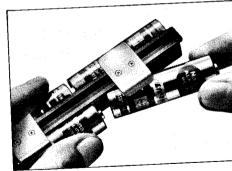
[3] After installing the batteries in the battery case, insert it into the battery compartment. Insert the case in the direction shown by the diagram in the battery compartment.
