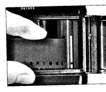
**5** Press the shutter release to take dummy exposures until the sprockets fit into the film perforations. Make sure that the sprockets fit into the performations, then close the camera back.
