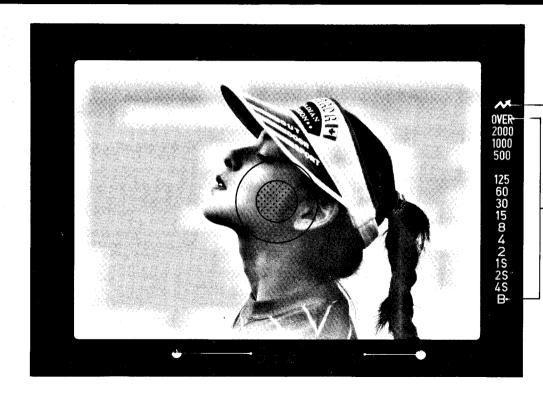
exposure data is given by means of an LED clay system. The display is turned on by pressing exposure check button, staying on continuously 6 seconds. The LED display features a two-ge brightness control which automatically adjusts the prevailing lighting condition, intensifying when went and dimming when dark.
